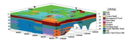
Lithostratigraphic model of Kolkata constructed from 654 boreholes showing the lithologic variation beneath Kolkata.
