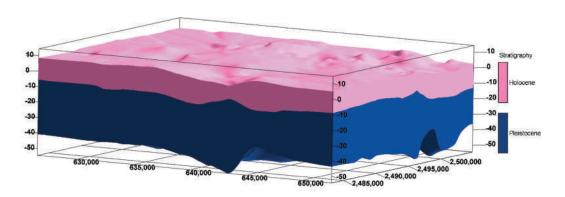
Stratigraphy model of the study region considering 654 boreholes' information illustrating the Holocene and Pleistocene sediment layers in depth.
