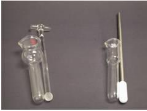
Figure . Two glass homogenizers used for shearing cells. The Dounce homogenizer (left) is manually operated and disrupts cells by forcing them between the pestle and tube wall. The Potter-Elvehjem homogenizer can be hand operated or attached to a motor. The pestle can be PTFE or glass.
