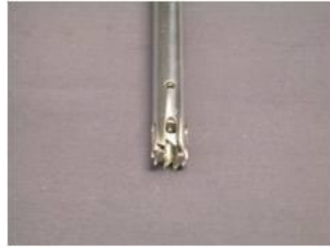
Figure. Top (upper) and side (bottom) views of a rotor/stator. The outer shaft (stator) remains stationary while the inner shaft (rotor) turns at speeds up to 20,000 rpm. Rotor/stators can be very effective on homogenizing powders and pills, but can generate only coarse homogenates when used on tougher tissues.
