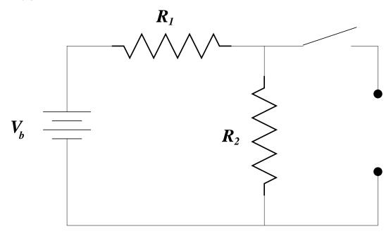
If we short circuit these terminals with a wire, a current  $I_{\rm SC}$  — the "short circuit" current — will flow. On the other hand, if we leave it open, there will be a potential difference — the "open circuit" voltage,  $V_{\rm OC}$  — between the terminals (equivalent to the potential drop over the resistor  $R_2$ ).
