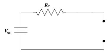
If you know what the big mess inside the "black box" is made out of, then you can figure out  $V_{\rm OC}$  and  $R_T$  as we did for the example above.
