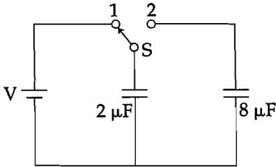
A capacitor of  $2 \mu\text{F}$  is charged as shown in the diagram. When the switch S is turned to position 2, the percentage of its stored energy dissipated is :
